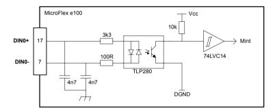
Figure 26 - General purpose digital input circuit
